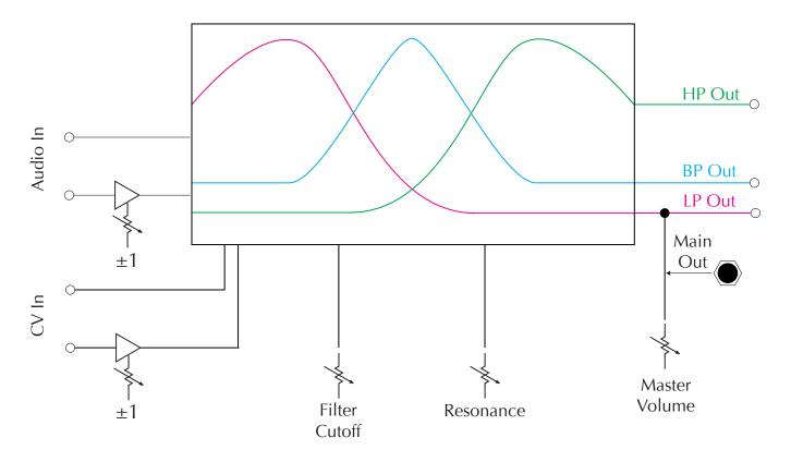
The filter has  $\pm 1$  attenuators on one audio input and one CV input. A  $\pm 1$  attenuator is like a bidirectional volume control—no signal goes through in the middle position; at fully clockwise, what came in goes out; at fully counter-clockwise, -1 what came in goes out.
