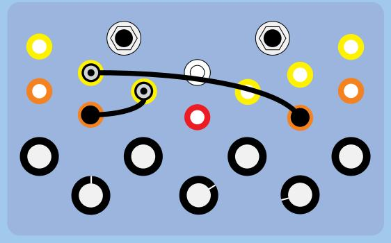
Experiment with different settings of the two oscillator pitch controls, and the master volume. The tone you hear is a complex function of the pitches of the two oscillators, and the distorting effect of the master volume further alters the harmonic content. You'll hear a wide range of clangorous tones.
